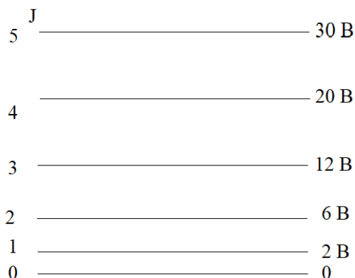
Fig.2 Allowed Rotational energy levels of a Rigid Atomic molecule
